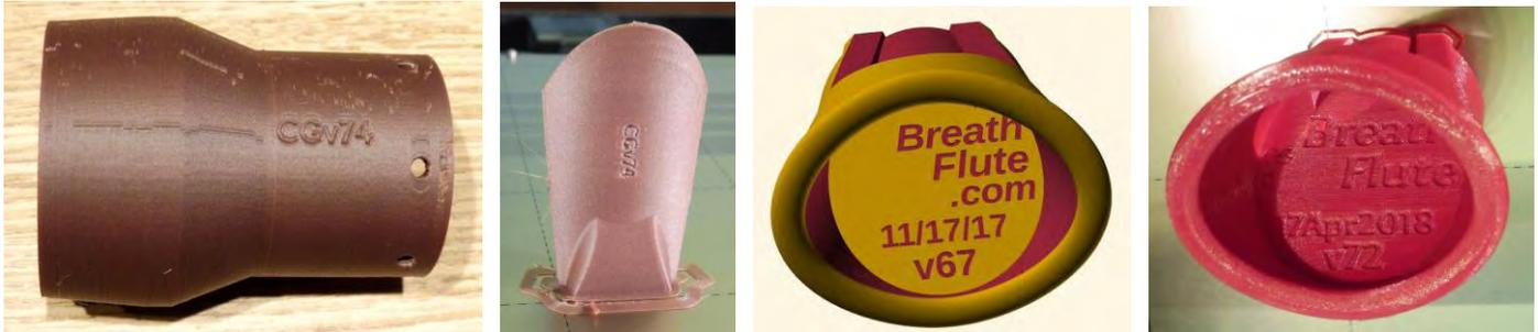
The **Foot** component is inscribed on the outside with the version and **XYExpand** parameter setting, since this is a test-only component. This is shown at the right for the v75 **Foot** component with an **XYExpand** setting of 005.
